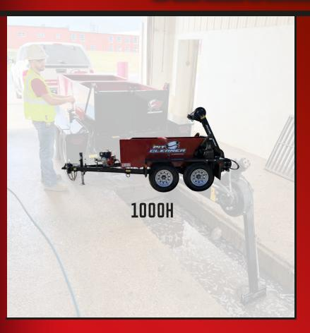
THE RING-O-MATIC CLAMSHELL PIT CLEANER LINE STARTED BACK IN 1960. THE CLAMSHELL DESIGN ALLOWS THE CONTRACTOR / CARWASH OWNER TO REMOVE THE MUD AND GRIME WHILE LEAVING THE WATER BACK IN THE PIT. THE 1000H HAS MADE IT SIMPLE FOR CAR WASH OWNERS TO SAVE MONEY ON WASTE REMOVAL. THIS TRUSTED MACHINE HAS PROVEN ITS PERFORMANCE FOR 60 PLUS YEARS NOW. CONTACT OUR SALES TEAM AND ORDER YOURS TODAY!
